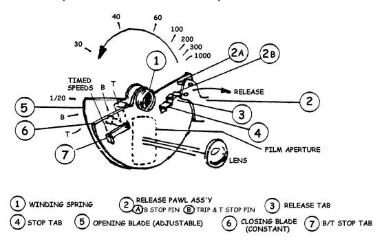
When the release is pressed, pawl 2 moves sideways as indicated, allowing tab 3 to pass. The disc spins freely for about 350° until stop tab contacts stop pawl (not shown in diagram). This pawl is linked to the winding mechanism, so that it releases and allows the disc to proceed on to pawl 2B just as the shutter spring is fully rewound. This operation is identical at all timed speeds, only the slit width being variable.
